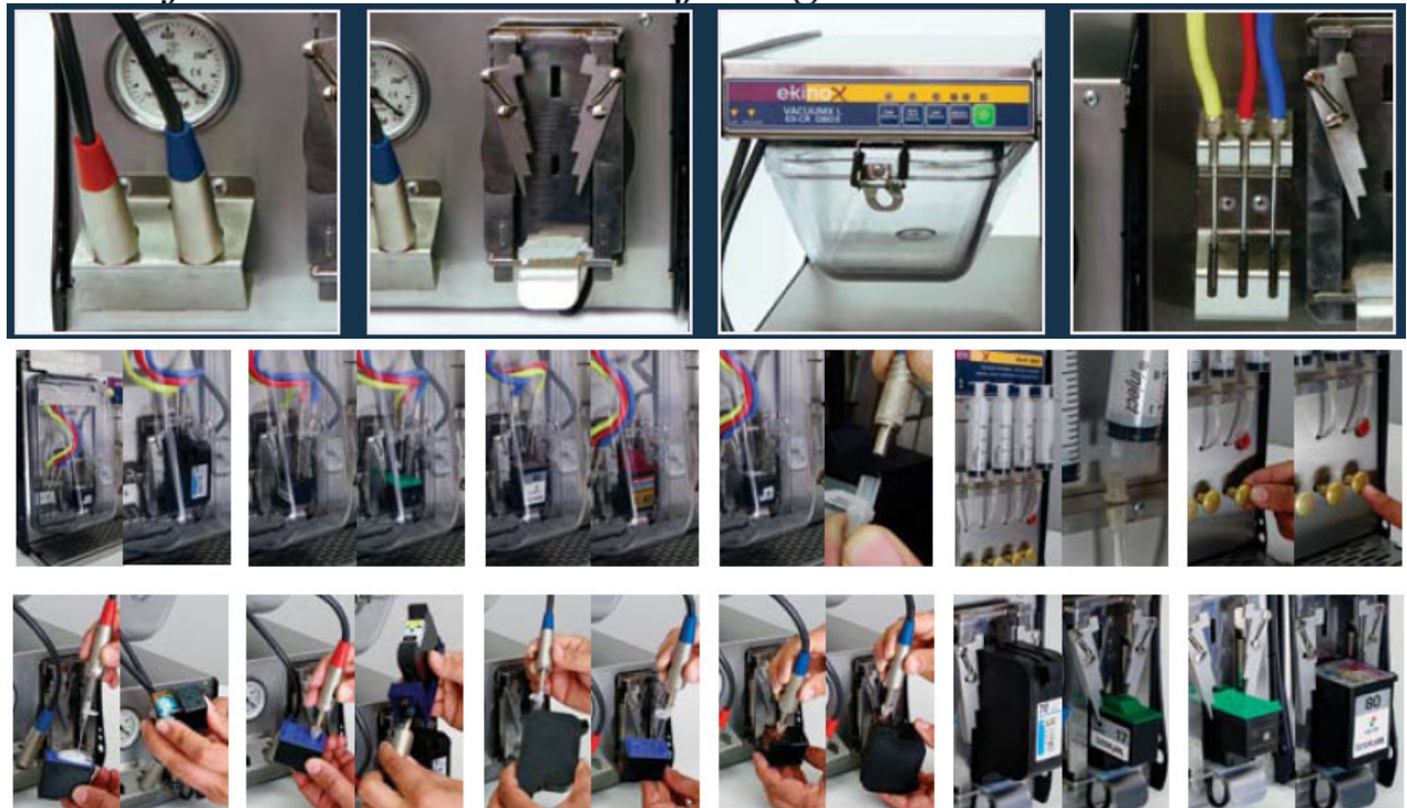
Powerful vacuum - Manuel filling with Vacuum Chamber.
